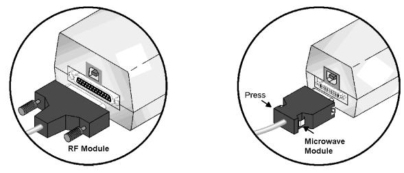
Figure 2-4 Parallel Port Connection to Module
