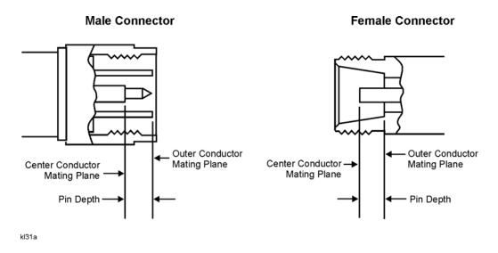
Light burnishing of the mating plane surfaces is normal, and is evident as light scratches or shallow circular marks distributed more or less uniformly over the mating plane surface. Other small defects and cosmetic imperfections are also normal. None of these affect electrical or mechanical performance. If a connector shows deep scratches or dents, particles clinging to the mating plane surfaces, or uneven wear, clean and inspect it again.
