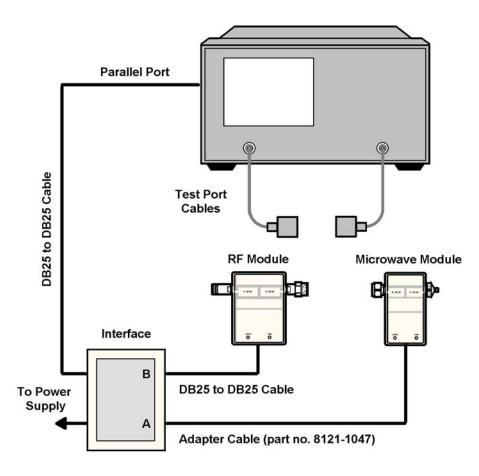
Preparing ECal for Use Connecting and Disconnecting ECal Module
