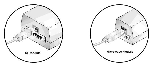
Figure 2-3 USB Connection to PNA or ENA Analyzer
