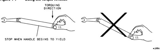
Figure 4-7 Using the Torque Wrench
